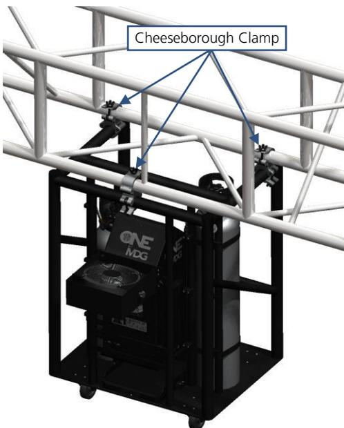
We recommend using **three** T57100 Series Cheeseborough clamp from Doughty Engineering with a **Safety Work Load of 750 kg (1650 lbs)** per clamp
